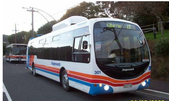
Prototype low floor trolley bus for Wellington by Designline. [Photo: G. Inwood]
