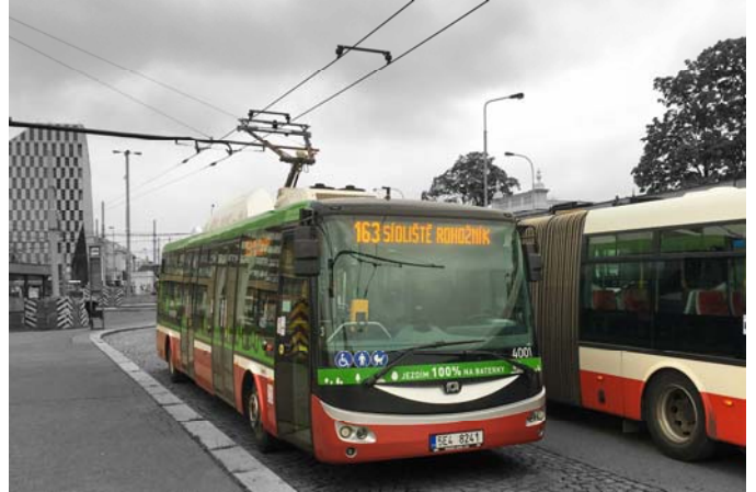
Prague's new electric buses charge under twin overhead trolley wires using a pantograph along a portion of their route; the remaining portion of the route is covered using the stored energy from traction batteries. [Photo courtesy DPP]
