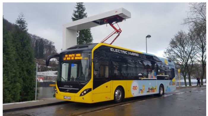
Volvo Battery Hybrid Bus docked at an ABB OppCharge charger. [Photo AB Volvo]
