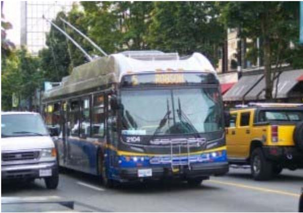
A modern low-floor trolley in service in Vancouver. Same chassis as diesel New Flyer ETS buses.
