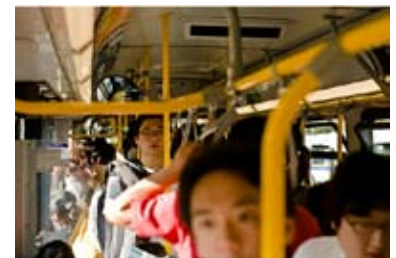
Figure 12. The crush capacity for articulated diesel buses in Vancouver, BC (above) is approximately 100 passengers. Demery & Higgins (2003) found that peak occupancy for buses is less than 3 passengers per meter compared to 4-5 passengers per meter for rail. Below is a picture of a modern streetcar at peak capacity.
