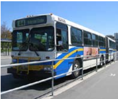
Figure 6. Shows an articulated diesel bus in service in Vancouver, BC with an energy efficiency of 4.25 passenger-miles per kWh.
